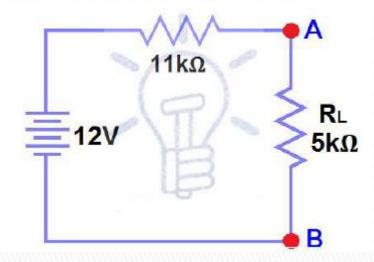
Now apply the last step. calculate the total load current & load voltage
