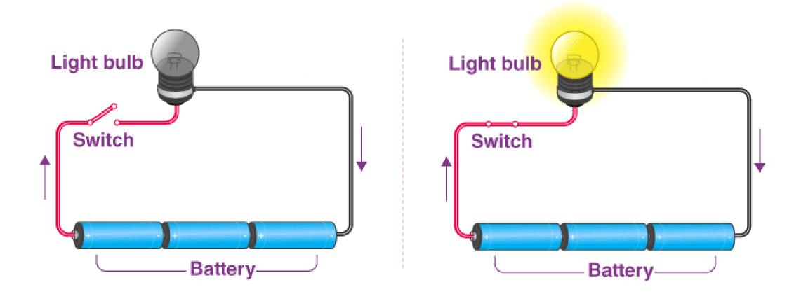
Connect the wires to the bulb and connect one end of the wire to the battery. Notice what happens, there won't be any change in the bulb, but when you connect the free wire to the battery and complete the circuit, you will notice that the bulb starts glowing. Therefore the circuit must be completed for the current to flow.
