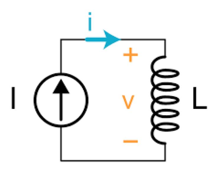
• Inductor stores Energy in a Magnetic field when electric current flowing through it
