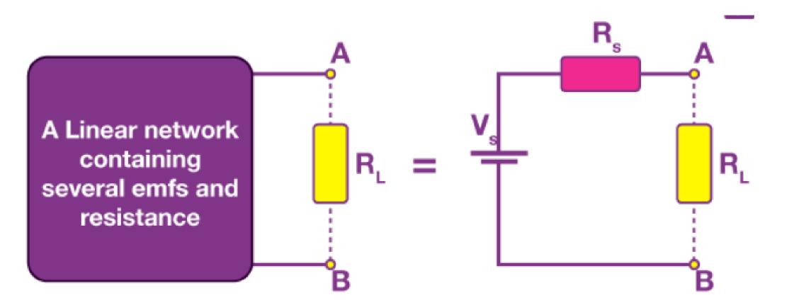
A Thevenin equivalent circuit is shown in the image. In the image, we see that multiple resistive circuit elements are replaced by a single equivalent resistance  $R_s$  and multiple energy sources by an equivalent voltage source  $V_s$ .
