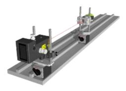
The straightness application is measured in two axis, where the laser beam is used as reference. The deviation in distance between the laser beam and the measurement object is measured in two or more positions with the use of a receiver.
