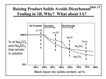
Since the product solids content from the 1B body is well above the transition point from burkeite to dicarbonate crystallization, there will be a substantial population of dicarbonate crystals in the liquor. Dicarbonate will be able to crystallize on the suspended crystals. The high degree of supersaturation needed for primary nucleation and subsequent fouling will never be reached.
