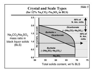
The second important point from Slide 5 is that, as evaporation of black liquor proceeds, the crystals produced can change from burkeite to dicarbonate. This happens because burkeite is sulfate-rich. As burkeite
