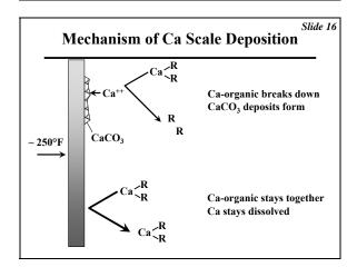
Mills with displacement batch pulping often have much more severe problems with CaCO<sub>3</sub> fouling in their evaporators. In these mills, the fouling occurs at lower temperatures, sometimes where the product liquor temperature is below 212°F (100°C). The reason is that soluble calcium-organic-bound calcium is extracted from wood chips by weak black liquor, which never is subjected to high temperature in a digester which reduces its fouling tendency [4].
