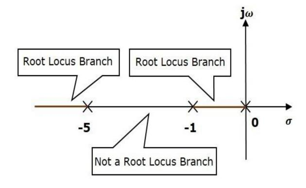
The three poles are located are shown in the above figure. The line segment between s=-1s=-1 and s=0s=0 is one branch of root locus on real axis.
