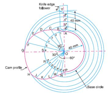
(b) Profile of the cam when the line of stroke of the follower is offset 20 mm from the axis of the cam shaft
