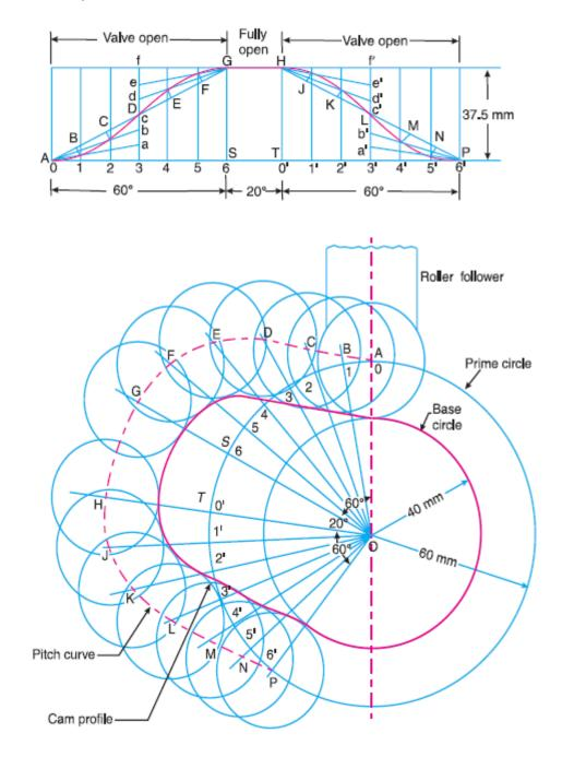
**Problem 5.** Draw the profile of the cam when the roller follower moves with cycloidal motion during out stroke and return stroke, as given below:
