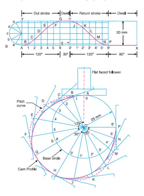
**Problem 4.** Design a cam for operating the exhaust value of an oil engine. It is required to give equal uniform acceleration and retardation during opening and closing of the value each of which corresponds to 60° of cam rotation. The value must remain in the fully open position for 20° of cam rotation.
