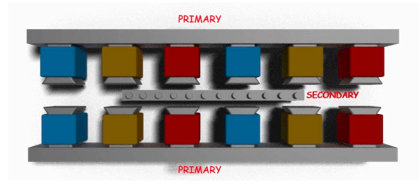
There is another variant of LIM also being used for increasing efficiency known as the Double Sided Linear Induction Motor or DLIM, as shown in the figure below. It has primary on either side of the secondary, for more effective utilization of the flux from both sides.
