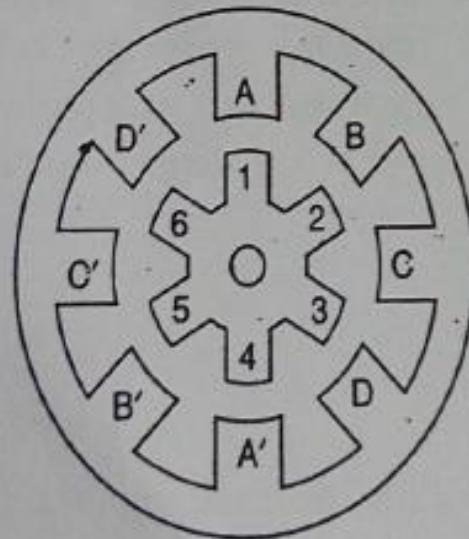
Fig. 1.3 Rotor position when phase A is excited
