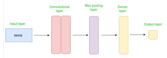
The Convolutional layer applies filters to the input image to extract features, the Pooling layer downsamples the image to reduce computation, and the fully connected layer makes the final prediction. The network learns the optimal filters through backpropagation and gradient descent.
