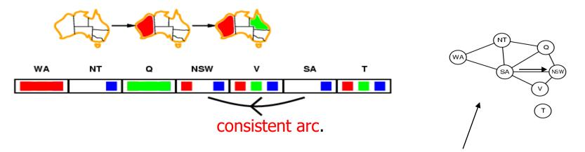
constraint propagation propagates arc consistency on the graph.
