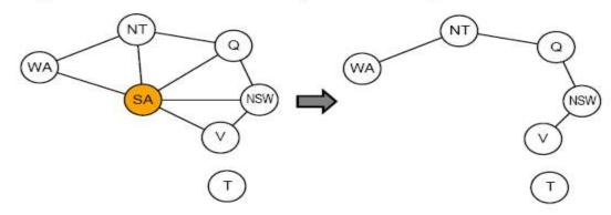
Cutset conditioning: instantiate (in all ways) a set of variables such that the remaining constraint graph is a tree
