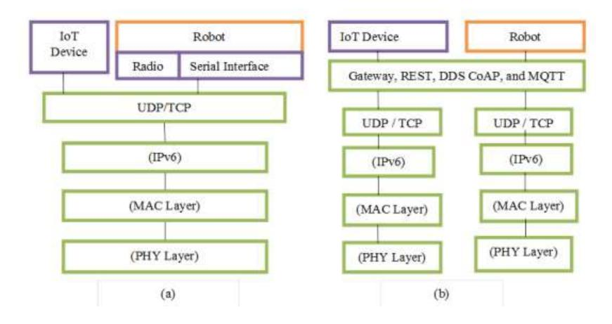
. (a) Robot acting like a node and (b) Robot acting like a client in IoT.
