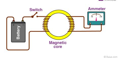
The experiment is not very complex. When a battery is disconnected, no electricity flows through the wire. Hence, no magnetic flux is induced in the iron (Magnetic
