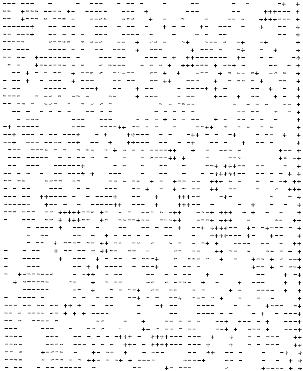
Figure 5-11. Sign map generated for the 3 x 3 filtered image of the sphere taking into consideration the magnitude of the depth value at a particular pixel and its neighboring pixel.
