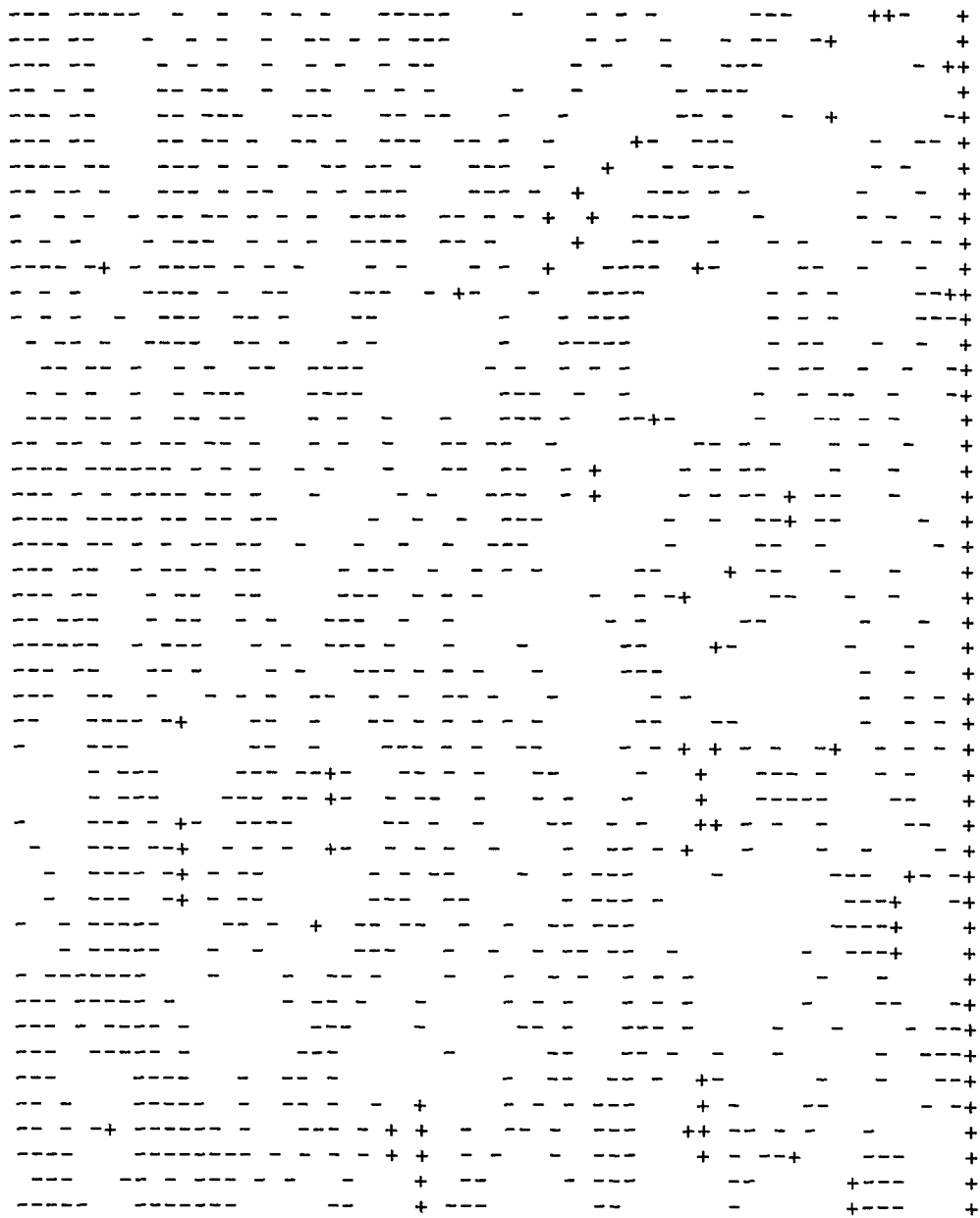
Figure 5-12. Sign map generated for the 5 x 5 filtered image of the sphere taking into consideration the magnitude of the depth value at a particular pixel and its neighboring pixel.
