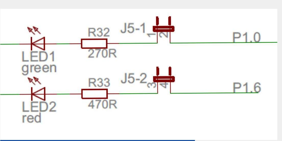
An LED can be connected directly to the MSP430 pin.
