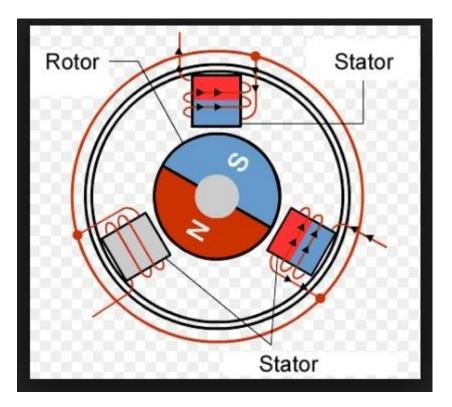
Normal motor shafts can move freely but the stepper motor shafts move in fixed repeatable increments.
