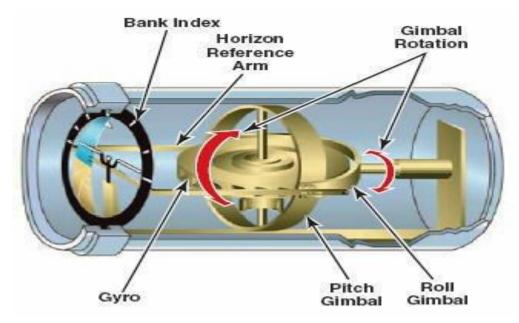
Gyroscopes play a crucial role in aircraft for maintaining orientation and stability, especially when external visual references are limited or unavailable. Here's how gyroscopes are used in various aircraft instruments:
