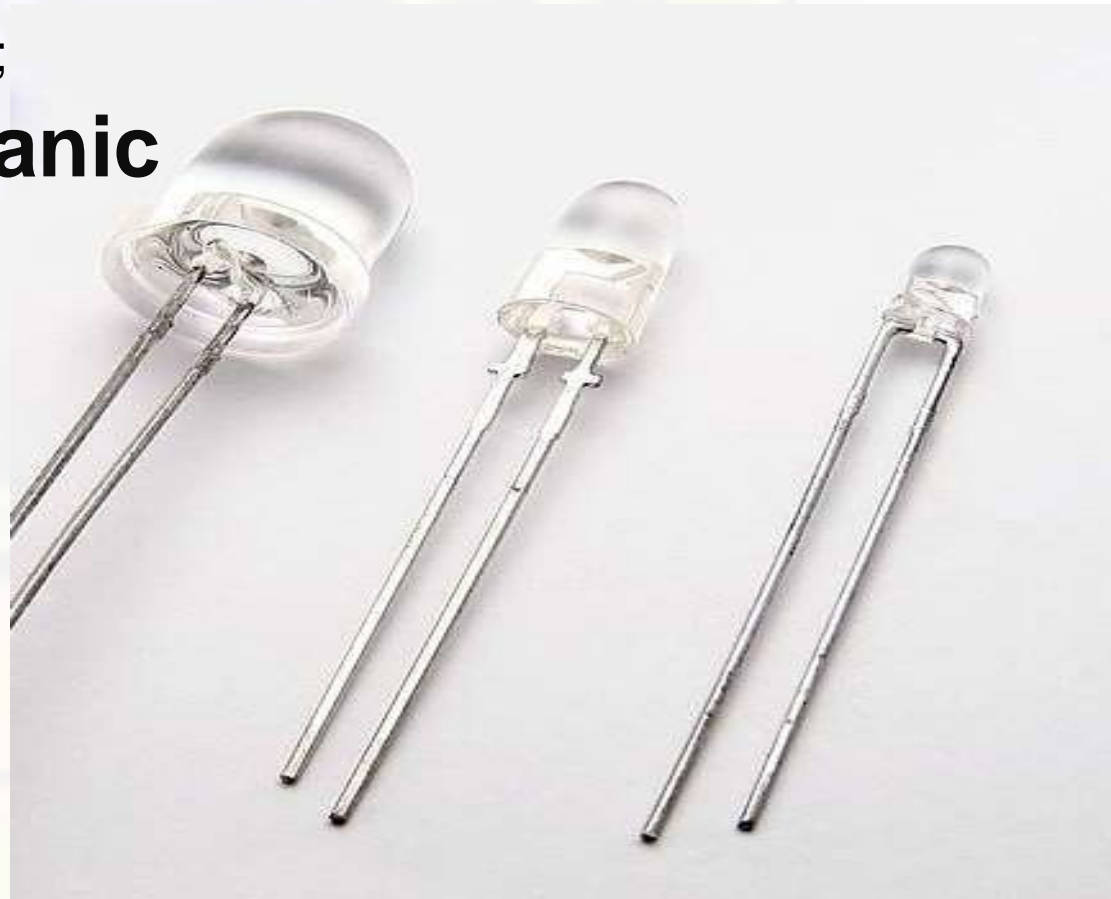
Different size of LEDs : 8 mm, 5 mm and 3 mm.
