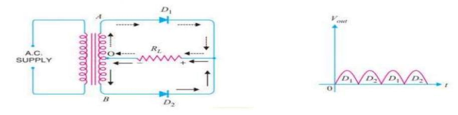
Circuit has two diodes D1, D2 and a centre tap transformer.
