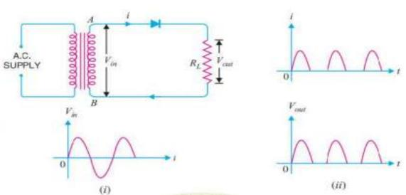
conducts no current through diode during positive half cycle only.
