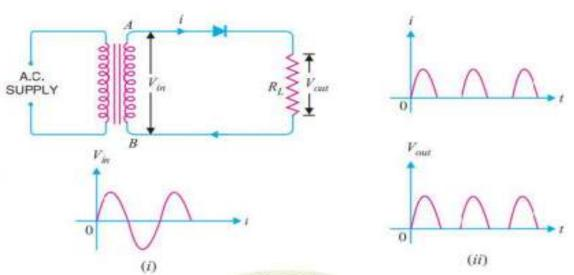
conducts no current So, current flows through diode during positive half cycle only.
