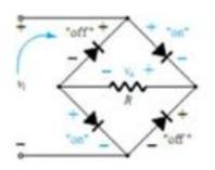
>During first half cycle D1 and D3 are conducting while D2 and D4 are in the "off" state.
