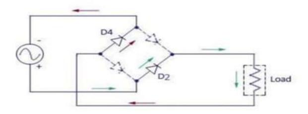
➤ During 2<sup>nd</sup> half cycle D2 and D4 are conducting while D1 and D3 are in the "off" state.
