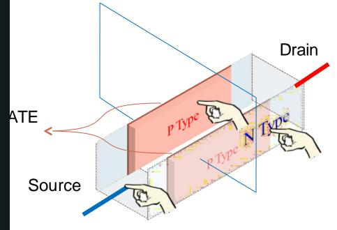
Fig 3. Construction of N Channel FET
