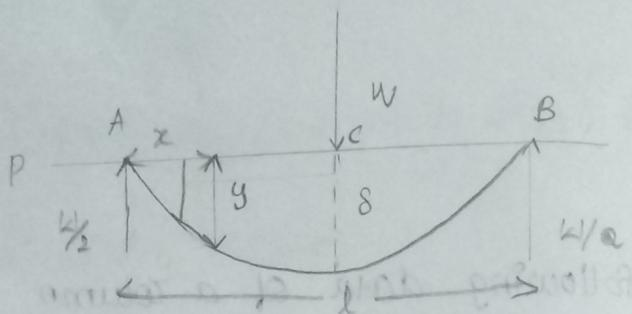
columns having transverse load in addition to the axial compressive load are termed as b.c.
