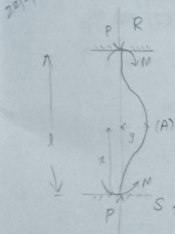
Consider a column R.S of length  $l$  and uniform cross sectional area  $a$  carrying a vertical load  $P$  at both ends. If the column is fixed at both of its ends due to application of load  $P$  the column will deflect as shown in figure.
