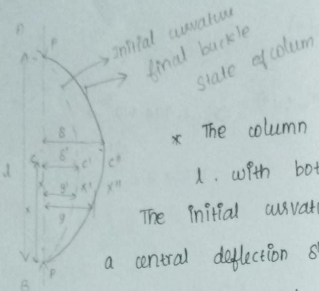
\* The column AB with length  $l$ , with both ends pinned.
