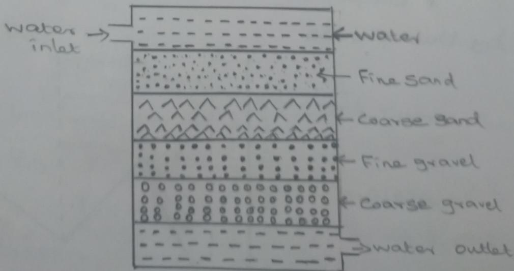
\* It is the process of removing bacteria, colour, taste, odour and suspended particles, by passing the water through filter beds containing fine sand, coarse sand and gravel.
