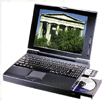
Maximum luminosity: 50% of CRT as 50% of light is blocked by the upper polarizer.
