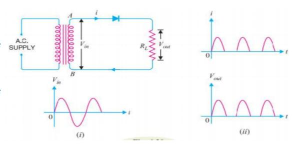
conducts no current flows through diode during positive half cycle only.
