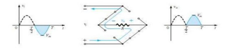
➤ During period t=T/2 to t=T D1 and D4 are conducting while D2 and D3 are in the "off" state.
