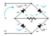
During period t=0 to t=T/2 D2 and D3 are conducting while D1 and D4 are in the "off" state.
