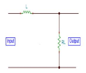
This type of filter is also called choke filter. It consists of an inductor L which is inserted between the rectifier and the load resistance R<sub>L</sub>. The rectifier contains A.C components as well as D.C components. When the output passes through the inductor, it offers a high resistance to the A.C component and no resistance to D.C components. Therefore, A.C components of the rectified output is blocked and only D.C components reached at the load.
