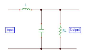
In inductor filter, the ripple factor is directly proportional to the load resistance. On the other hand in a capacitor filter, it is varying inversely with the load resistance. Hence if we combine the inductor filter with the capacitor the ripple factor will become almost independent of the load filter. It is also known as inductor input filter, choke input filter, L input or LC-section.
