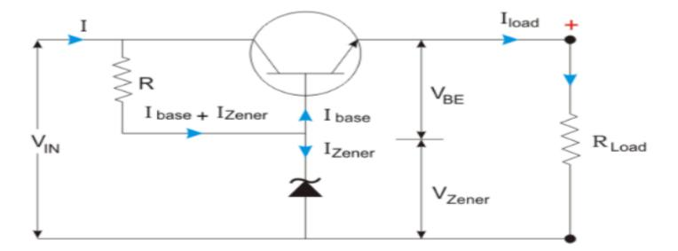
$V_{OUT} = V_{Zener} + V_{BE}$
