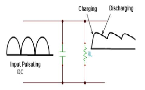
In this filter a capacitor is connected across the load during the rise of voltage cycle it gets charge and this charge is supply to the load during the fall in the voltage cycle. This process is repeated for each cycle and thus the repel is reduced across the load. It is shown in the above Figure. It is popular, because of its low cost, small size, less weight and good characteristics. Useful for load up to 50mA as in transistor radio battery eliminators.
