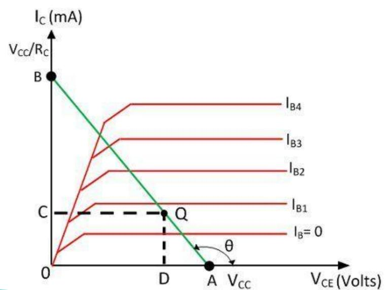
• 1. The collector-emitter voltage VCE is maximum when the collector current IC = 0 then from the equation (1) we get,  $V_{CE} = V_{CC} - 0 \times R_C$
