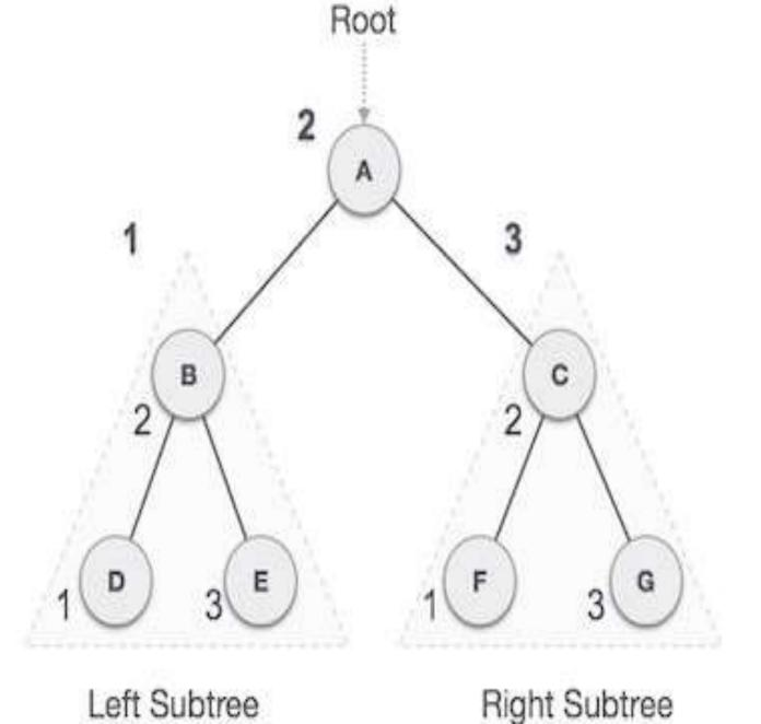
If a binary tree is traversed in-order, the output will produce sorted key values in an ascending order.
