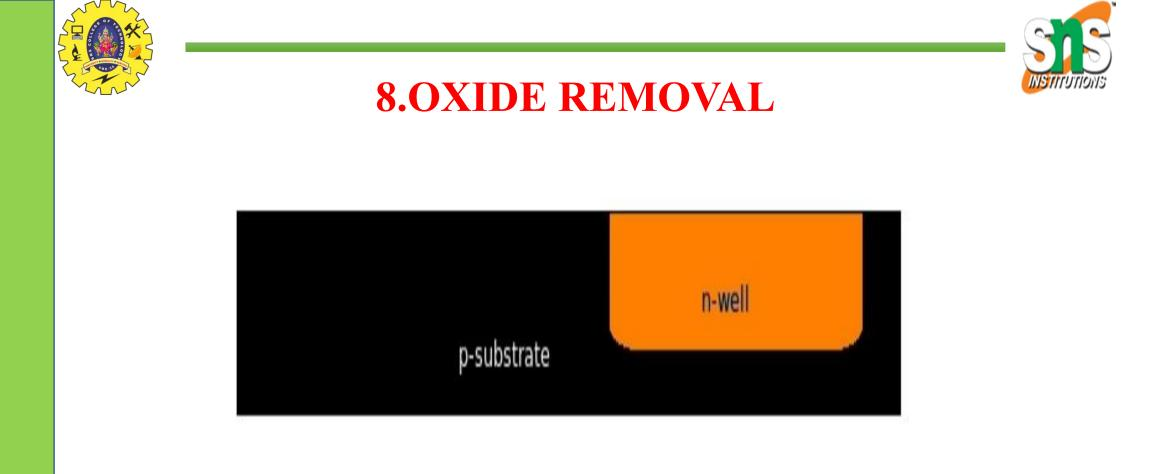
The remaining oxide is stripped with HF acidThis leaves the exposed wafer with the n-well formed
