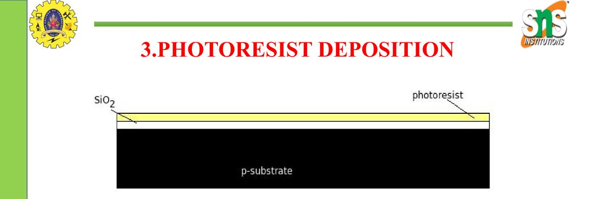
The photoresist is deposited throughout the waferThe PR has to be patterned to allow formation of the well
