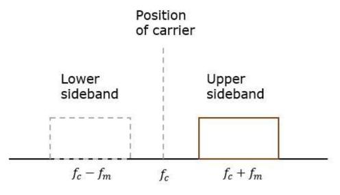
Carrier and a sideband are suppressed and a single sideband is allowed for transmission
