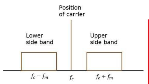
Both the sidebands in the right side of the image contain the same information. The transmission of such a signal which contains a carrier along with two sidebands, can be termed as **Double Sideband Full Carrier** system, or simply **DSB-FC**. It is plotted as shown in the following figure. However, such a transmission is inefficient. Two-thirds of the power is being wasted in the carrier, which carries no information.
