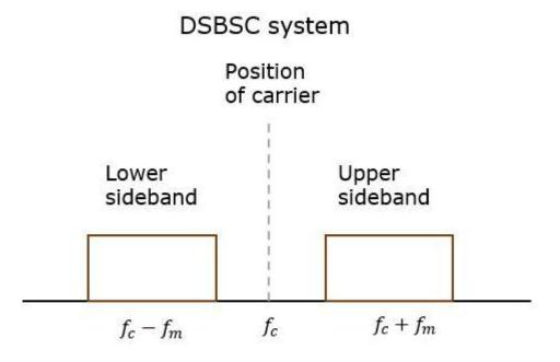
Carrier is suppressed and sidebands are allowed for transmission
