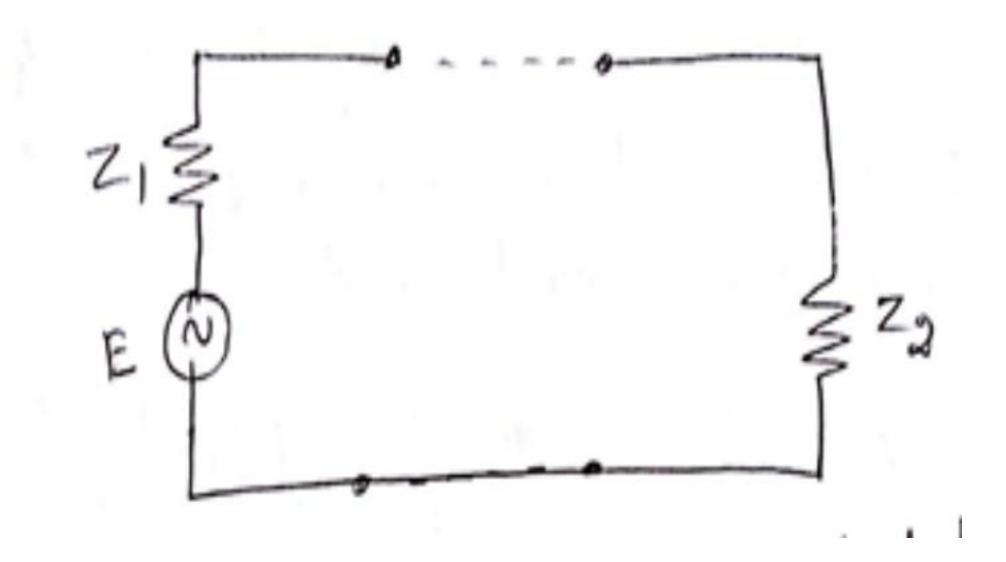
FIG. Generator of impedance  $\mathbf{Z}_1$  connected to load  $\mathbf{Z}_2$
